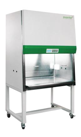
These cabinets have powerful exhausts that throw out air and filter the area making the environment free from any harmful bacteria or virus. One more category of these BSC is the laminar airflow category that works on a contradictory mechanism. This type of biosafety cabinet throws unfiltered air on the person and is not considered safe while working with pathogens. The biosafety cabinets are bifurcated into three classes.
